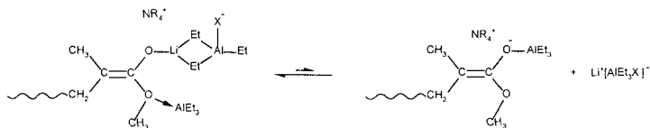
Scheme 2: Tentative dissociation of the active species in Scheme 1 into to a ester enolaluminate with \text{NR}_4^+ counterion and a \text{Li}^+[\text{AlEt}_3\text{X}]^- complex.
